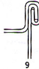
9 Completed Double Seam
