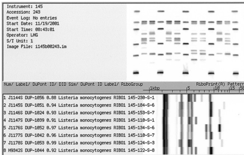
Fig. 13.1 RiboPrint ® patterns of Listeria monocytogenes isolates generated using DuPont Qualicon RiboPrinter ® system. The unprocessed TIFF image (top right) shows ribotype patterns of 8 L. monocytogenes isolates (lanes 2,3,5,6,8,9,11,12). A molecular size standard is in lanes 1,4,7 and 10. The RiboGroup patterns and RiboGroup IDs of the patterns are displayed in the bottom panel of the RiboPrinter ® output.
