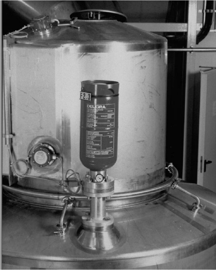
Fig. 16.19 Commercial explosion suppression system mounted on top of a cyclone (courtesy of Anhydro A/S).
