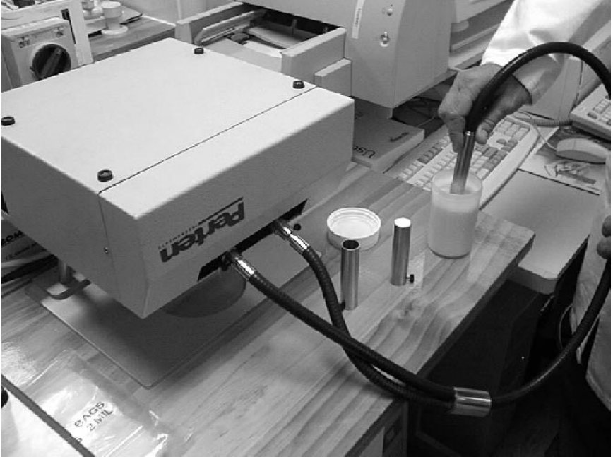
Fig. 13.4 At-line NIR determination of moisture, salt and fat in butter (Holroyd 2002).
